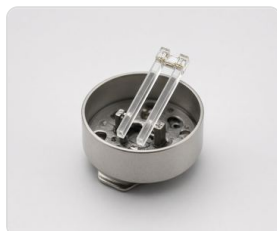
11. Quartz timing crystal (in the core)
